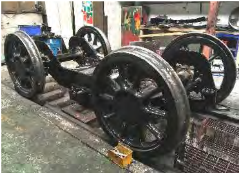
The front bogie is now completely refurbished and awaiting final assembly.
