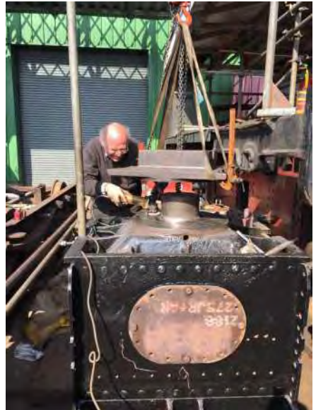
Above: Much easier to clean and paint these bottom pockets when the casting is upside down!
