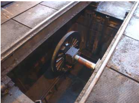
Leading and centre driving wheelsets are now in. The photos above show Ropley wheeldrop in use to locate the leading drivers.
