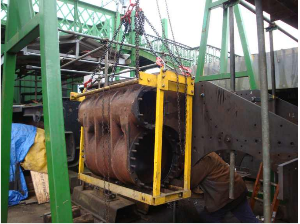
R/H cylinder block lifted on 499. Photo © ULS
