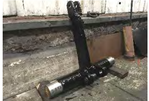
Brake weighshaft has been machined.
