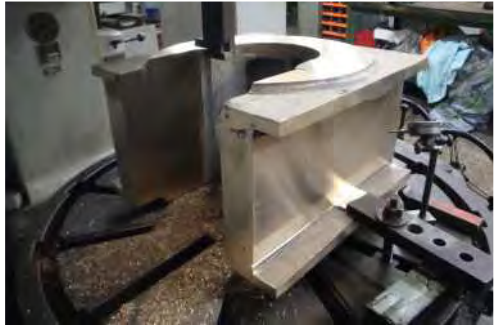
Four existing axleboxes and a new one have been completed. The second new box is machined and awaiting white-metalling.
