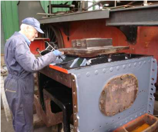
Above: Much easier to clean and paint these bottom pockets when the casting is upside down!
