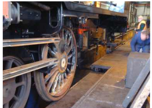
Leading and centre driving wheelsets are now in. The photos above show Ropley wheeldrop in use to locate the leading drivers.
