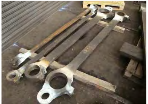
Wear in the bores on the coupling rods has been built up with weld.
