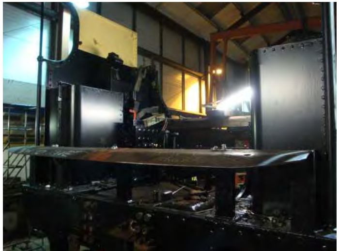
Inside of the cab freshly painted. Note the new tool boxes. © ULS
