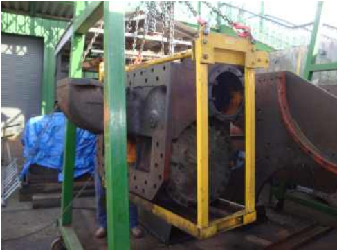
A case of déjà vu as 499s LH cylinder block is prepared for lifting. Photo © ULS
