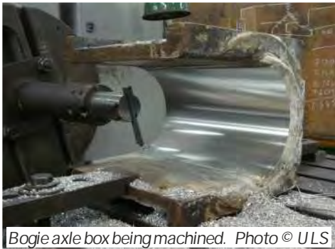
Bogie axle box being machined. Photo © ULS
