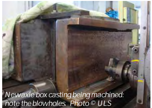
Bogie axle box being machined. Photo © ULS
